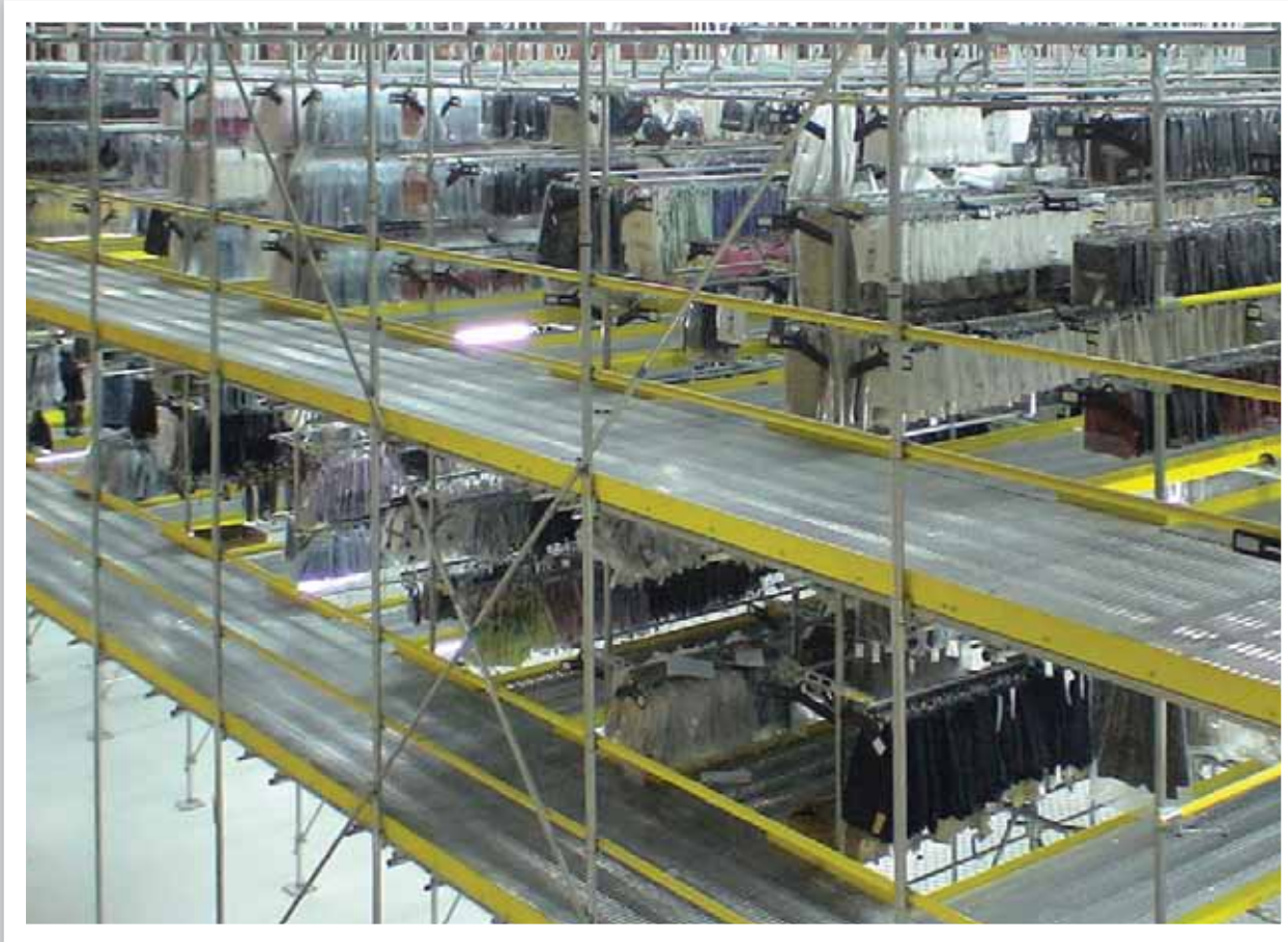
Garment handling equipment for production, processing, storage, picking and transportation of hanging and folded garments.
